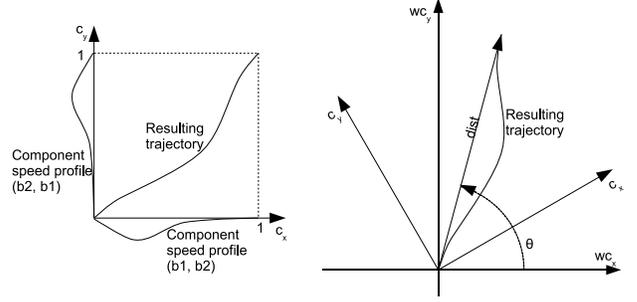
Fig. 2. Sketch of how the TBGs generate a hand non-linear trajectory. **Left:** example of trajectory generated by Eq. 5. **Right:** same trajectory after a rotation and scaling (see Eq. 6).
