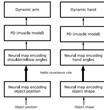
Fig. 6. The architecture of the grasping model, formed by four neural maps for reaching and grasping, PD muscle models, and a dynamic arm-hand model. Plain arrows refer to information flows whereas bold arrows represent connection weights trained on the basis of an Hebb rule.
