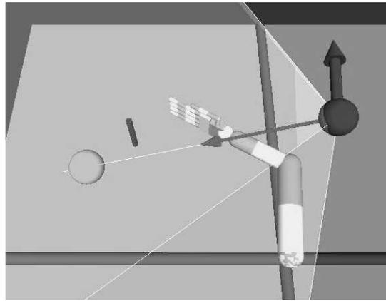
Fig. 1. The robotic setup used to test the models. The picture focuses on the north-west quadrant of the four working plane quadrants. The sphere with the arrows indicates the position of the eye (thin arrow: current gaze; thick arrow: camera up-vector). The sphere in front of the arm is the object that the robot tries to reach (first model) or grasp (second model: in this case it is the “big object” ). The cylinder represents the obstacle to be avoided (first model).
